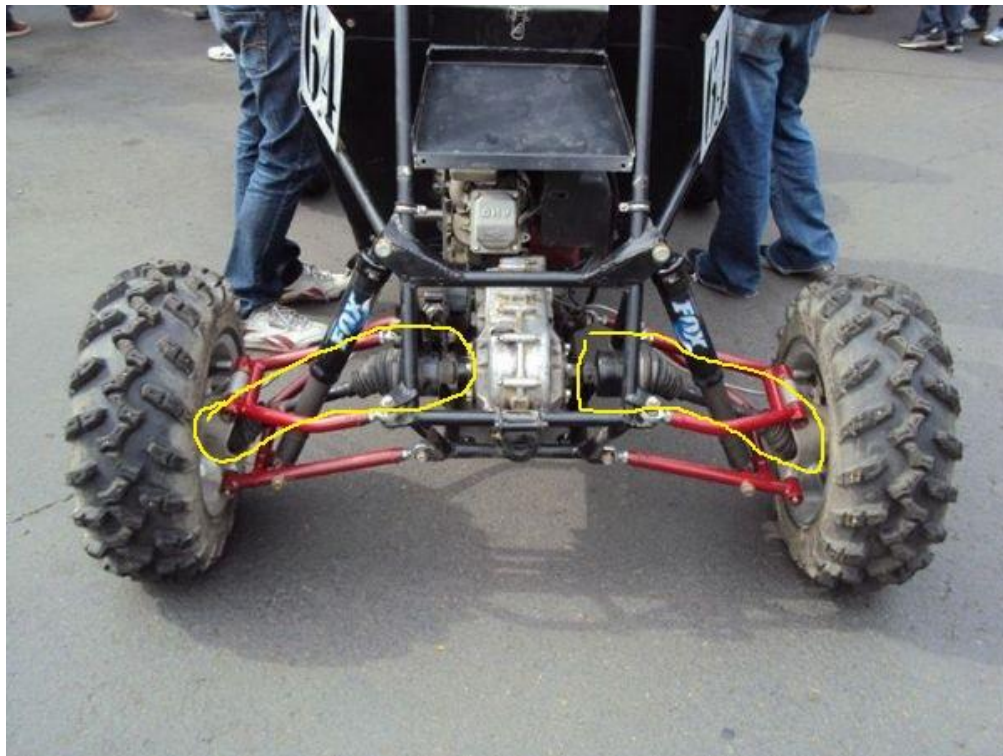
Figure 4 - Baja with independent axles (yellow circles). Courtesy of Pedro_UFPBaja, forums.bajasae.net.
