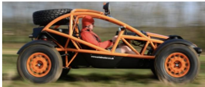
Figure 5 - A vehicle composed of a simple strutted frame. [2]
