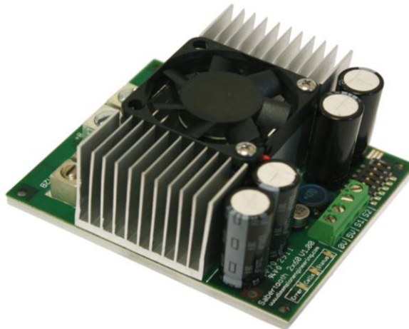
Figure 16c - Sabertooth Dual 60A Motor Driver.
