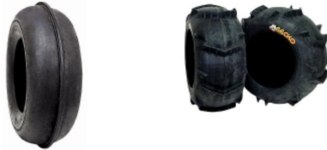
Figure 7 - A blade tire, left, and a paddle tire, right, shown [6]
